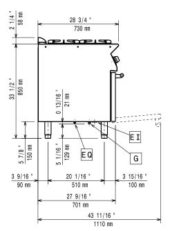
Electrical inlet (power) Gas connection
